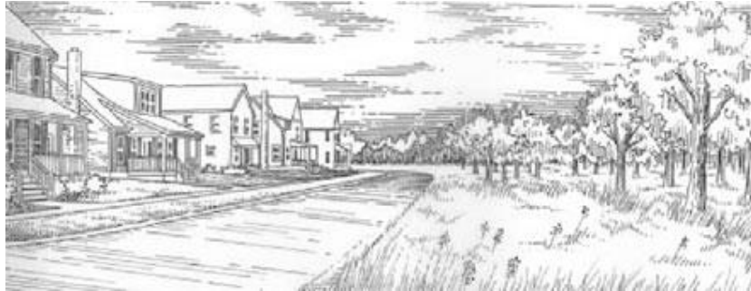
Figure 1705.B.3.a (example of a single loaded street)
