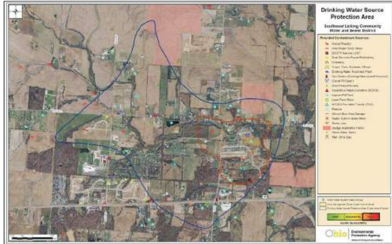
Map 12: Drinking water source protection area and potential contaminant source inventory (Source: Ohio Environmental Protection Agency).
